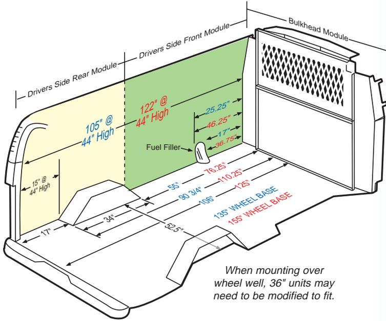
When mounting over wheel well, 36" units may need to be modified to fit.
