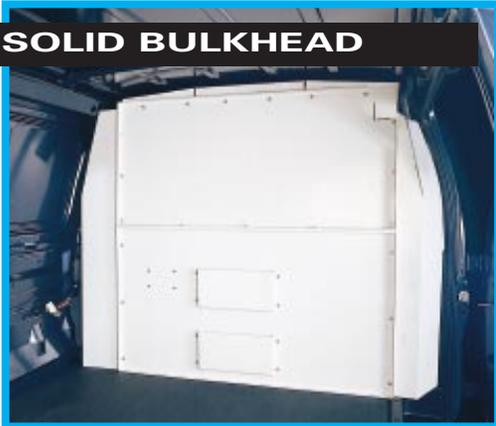
Solid Bulkheads offer the driver maximum protection from shifting loads.
