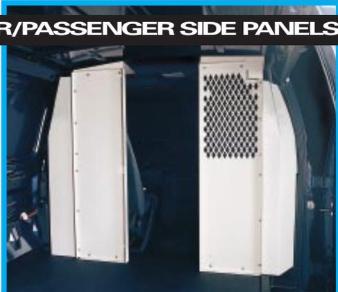
Single panels are available for the driver or passenger side or both. Used together, they leave a walk through.
