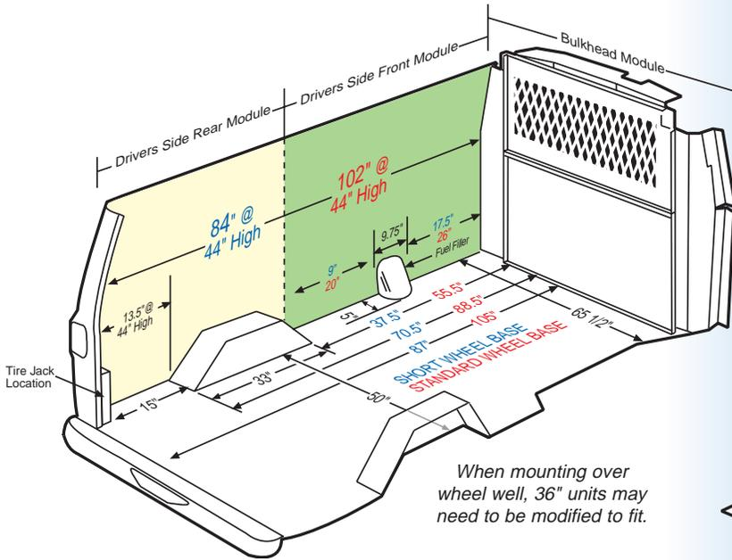
The dimensions shown in this guide refer to the 2003 model year full size Dodge Ram vans. Dimensions printed in blue refer to short wheel base vans, dimensions printed in red refer to standard wheel base vans. Dimensions printed in black are common to both. You should always measure your van carefully to make sure the equipment you choose will fit properly.
