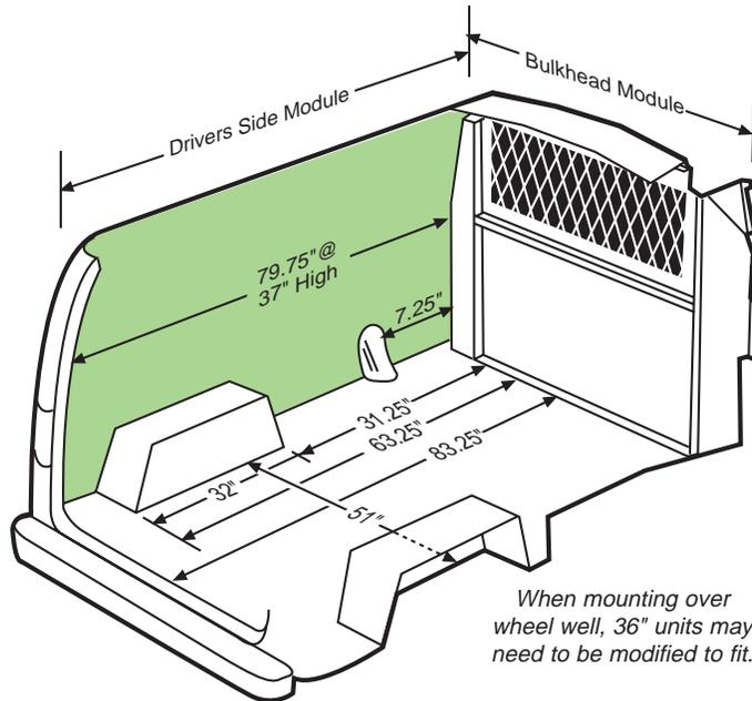
When mounting over wheel well, 36" units may need to be modified to fit.
