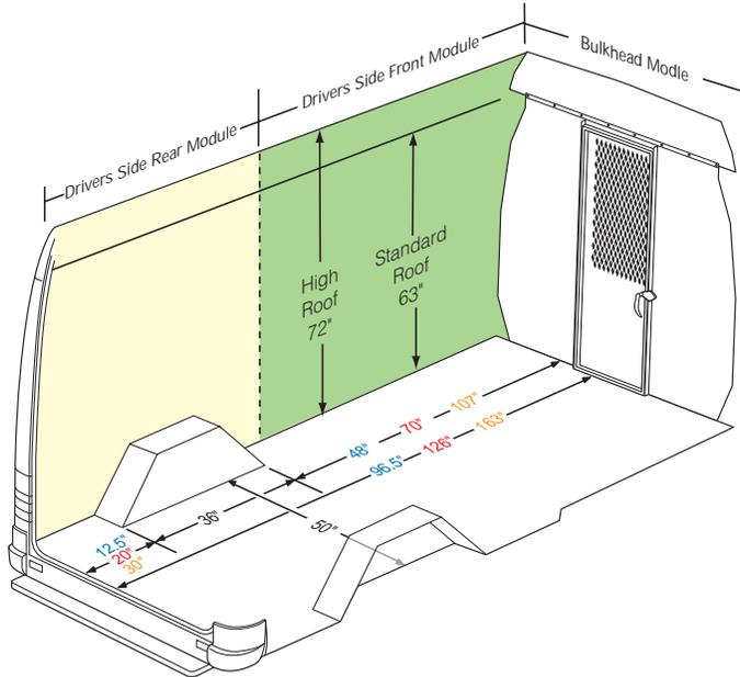
The dimensions shown in this guide refer to the 2003 model year Sprinter vans. Dimensions printed in blue refer to 118" wheel base vans, dimensions printed in red refer to the 140" wheel base vans and dimensions printed in orange refer to the 158" wheel base vans. Dimensions printed in black are common to all. You should always measure your van carefully to make sure the equipment you choose will fit properly.
