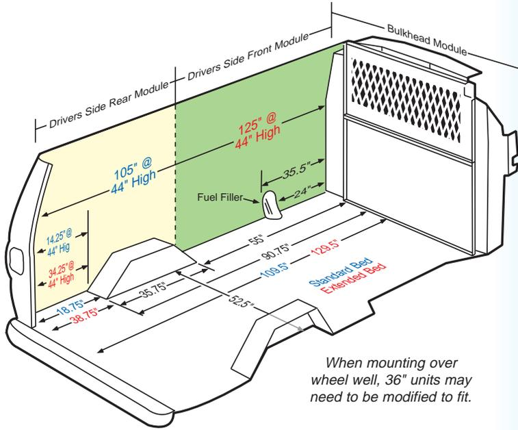
The dimensions shown in this guide refer to the 2003 model year full size Ford Econoline vans. Dimensions printed in blue refer to standard wheel base vans, dimensions printed in red refer to extended wheel base vans. Dimensions printed in black are common to both. You should always measure your van carefully to make sure the equipment you choose will fit properly.
